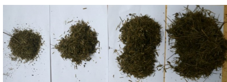
Tamis < 4 mm, 4-8 mm, 8-19 mm et > 19 mm
